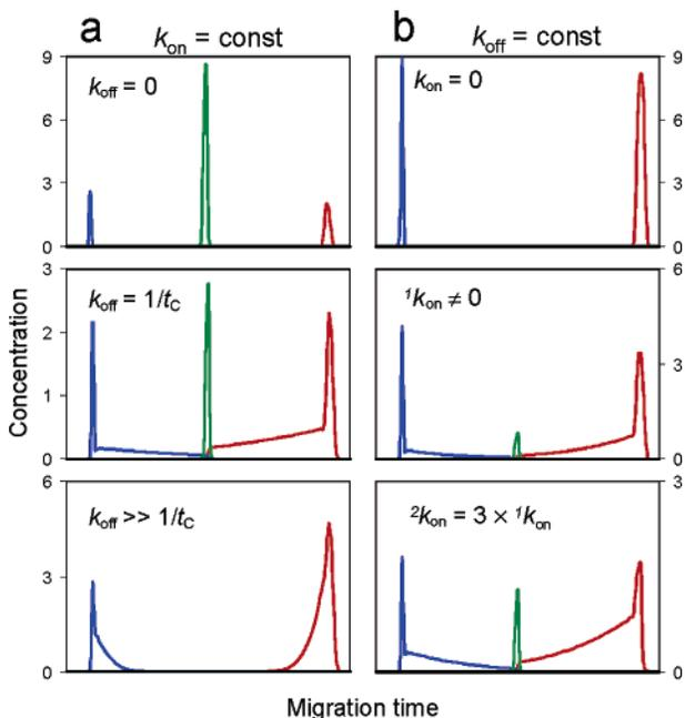
**Figure 2.** Simulated ppKCE electropherograms for constant  $k_{\text{on}}$  and three different  $k_{\text{off}}$ 's (panel a) and for constant  $k_{\text{off}}$  and three different  $k_{\text{on}}$ 's (panel b). Red, green, and blue colors correspond to  $A(t)$ ,  $C(t)$ , and  $B(t)$ , respectively.
