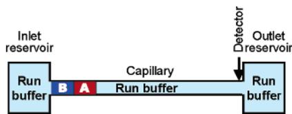
**Figure 1.** Schematic representation of initial and boundary conditions in ppKCE.
