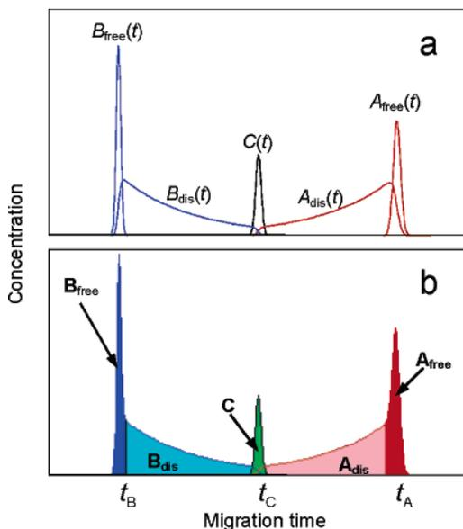
**Figure 3.** Panel a shows simulated ppKCE concentration profiles, with functions  $A(t)$  and  $B(t)$  being presented as a superposition of free and dissociated components (see equation 4). Panel b illustrates measurable parameters (areas of peaks and smears and migration times of A, B, and C), which are used for the determination of  $k_{\text{on}}$  and  $k_{\text{off}}$  without nonlinear regression analysis.
