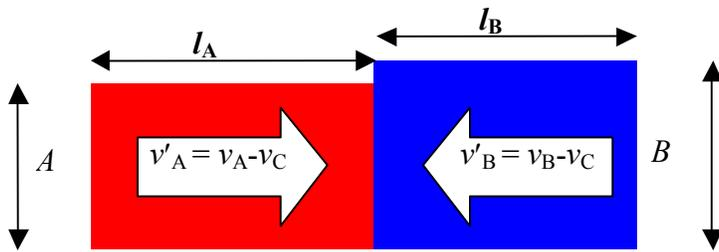
**Figure 1.** Graphic representations of 2 plugs interacting in the capillary. The heights of the rectangles correspond to concentrations of A and B in the plugs.
