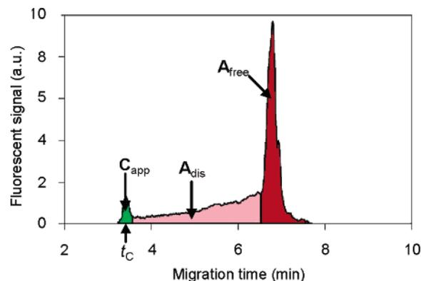
**Figure 4.** Experimental electropherogram for 200 nM SSB with 200 nM fluorescently labeled DNA interaction using ppKCE method. The areas used in analysis are color-coded: green for the complex, pink for the decay, and red for the unreacted DNA.
