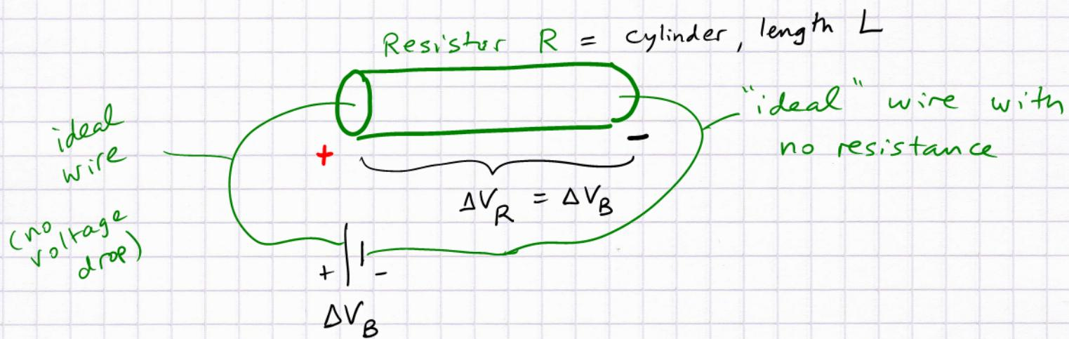
An electric field of strength  $E = \frac{\Delta V_R}{L}$  would push positive charges left  $\rightarrow$  right, i.e., it pushes conduction electrons right  $\rightarrow$  left.
