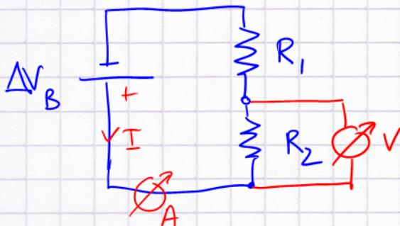
$$\Delta V_2 = R_2 \cdot I = \frac{R_2}{R_1 + R_2} \Delta V_B$$
