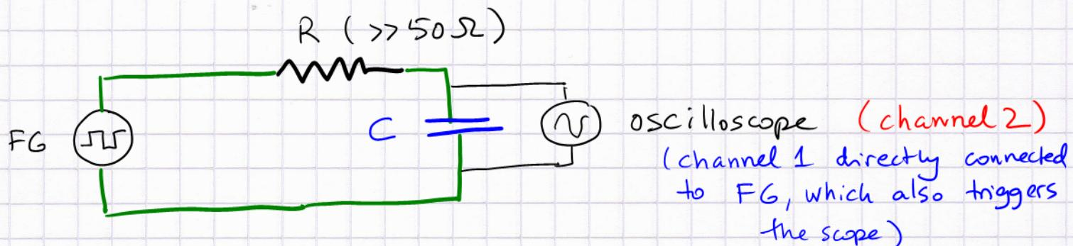
The oscilloscope records the voltage drop across the charging / discharging capacitor periodically in time
