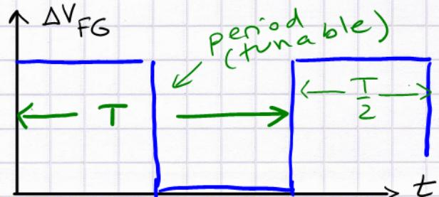
The function generator acts to mimick the "battery + switch" configuration. When the generator is low it acts as a "short" (really a  $50\Omega$  resistor).
