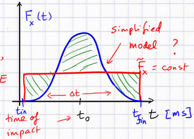
then deformed tennis ball decompresses + accelerates the ball in the opposite (upward) direction.
