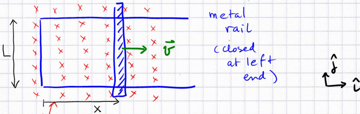
uniform  $\vec{B}$  field into the plane, from permanent magnets or from electro-magnets.  $\vec{B} = -B_0 \hat{k}$
