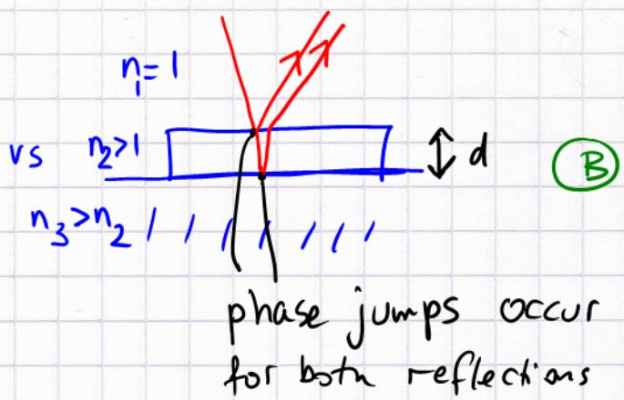
For a thin plate (film) in air the reflections from the front and bottom surfaces are different.
