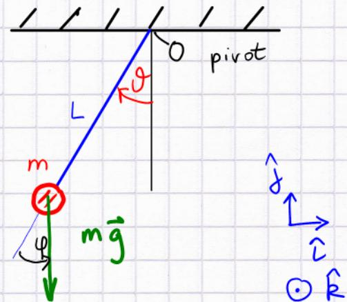
$$I_0 \alpha = I_0 \frac{d^2 \theta}{dt^2} = \tau_z \quad \leftarrow \text{gravitational torque about } O$$
